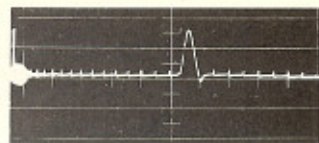
Fig. 5. Sweep magnifier on. 20 Microsecond Pulse.
