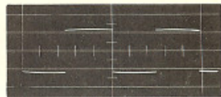
Fig. 2. 60 cycle square wave. Response of 2 Stage Vertical Amplifier.
